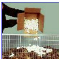
This loose-fill for packaging industry is made of foamed starch.
