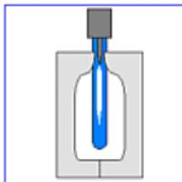
Used for hollow parts of all sizes. A tube of molten plastics is extruded into an open mould. The mould closes and thereby the bottom of the part welds.
