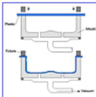
Well suited for larger plastic parts since tools investments are low. Also used for high volume production of e.g. disposable cups and chocolate packaging. The surface facing the mould has the best quality. Material thickness is difficult to control.
