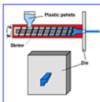
Profiles of all shapes can be produced. In an extruder the material is heated and continuously pushed by a rotating screw through a die with the shape of the profile. After the die, the profile is cooled by air or water and cut into desired lengths.
